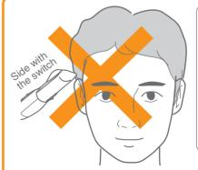
Do not use the trimmer switch side up as shown in the illustration on the left. This will result in cutting more than the desired length.
